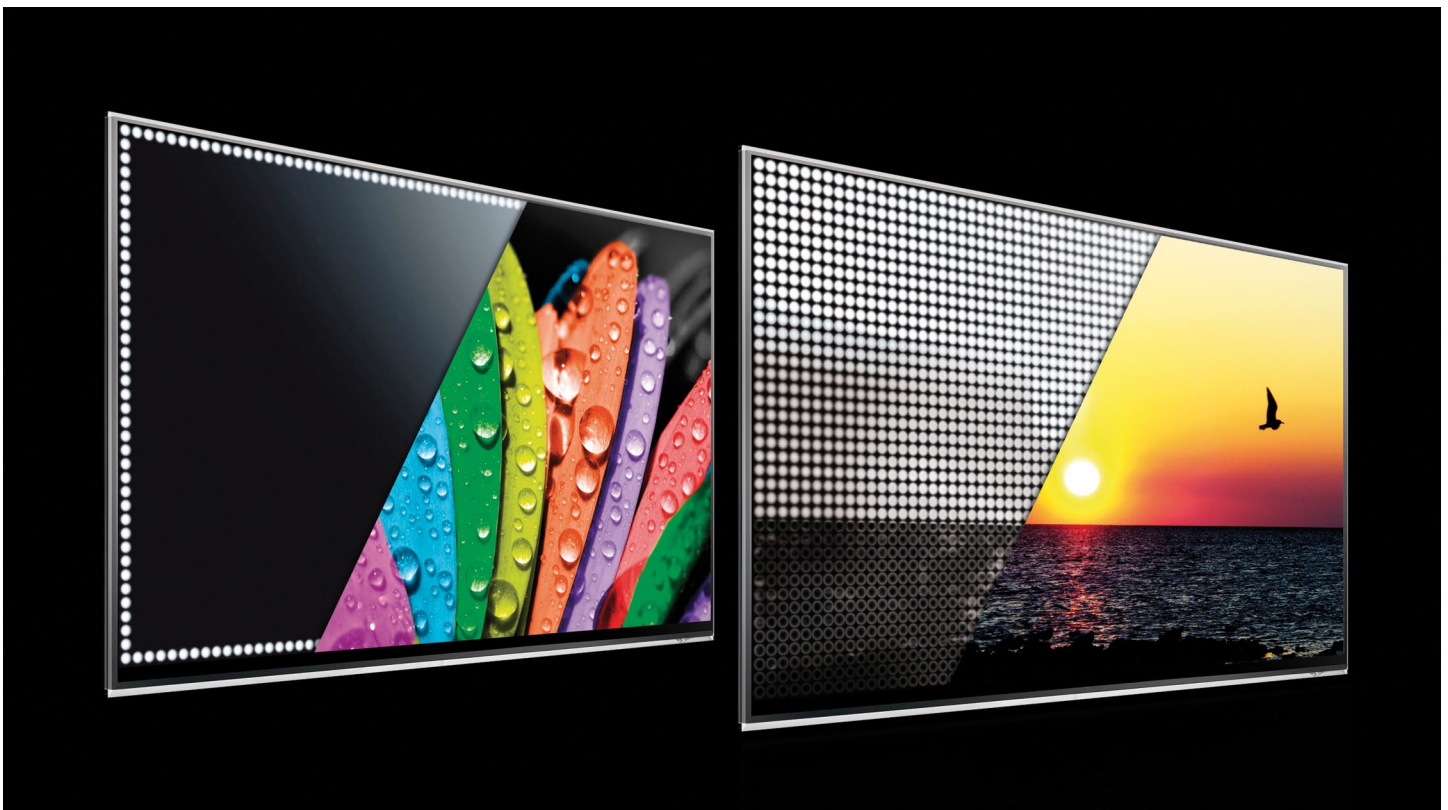
Figure 1 LCD TVs can adopt one of two arrangements for LED backlighting: indirect (edge light) (a) or direct (b).
